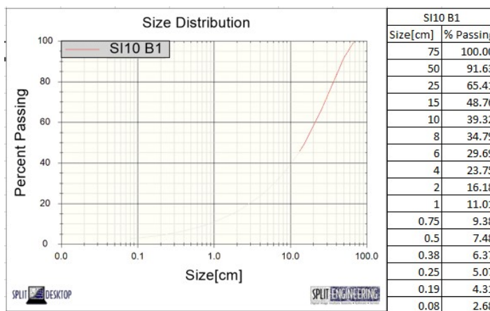
Gambar 14. Distribusi Fragmentasi Aktual Geometri III Blok B1 ( Split Desktop )
